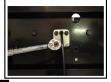
Place top plate over intermediate plate with dots facing toward the top. Make sure the shaft protrudes all plates.
