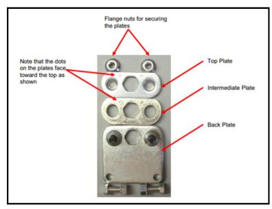
Note - FE rollers require one (1) bracket on cable end only.
