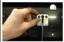
Install flange nuts and finger tighten.
