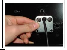
Place intermediate plate onto back plate over the studs, ensuring the depressions fit over the cones on the studs and the dots face toward the top.
