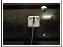
Fasten back plate to frame and tighten nuts to 2.6 lb-ft (3.5 Nm)
