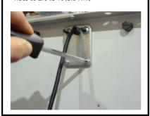
Place top plate over intermediate plate with dots facing toward the top. Make sure the shaft protrudes all plates.
