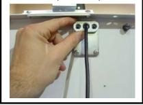
Alternately tighten nuts using a torque wrench set between 4.4 – 7.4 lb-ft (6 Nm – 10 Nm).
