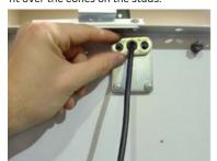
Install flange nuts and finger tighten.
