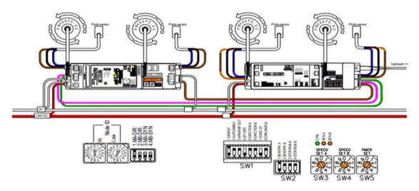
An HBM-604B-UL can exchange handshake signals with the IB-E03B and IB-E04F. Product will accumulate at the last zone before the IB card. When sensor A is blocked on the HBM-604B-UL, it sends the sensor out signal to the IB. The IB then sends a force run signal to the HBM. If an HBM-604B-UL has an error, the error output signal is pulsed from the HBM-604B-UL to the IB card which can determine the error condition and bring it to upper level Ethernet communication.
