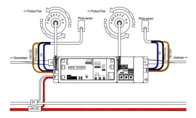
This configuration (factory set) is the standard set-up for any zone that is not specifically an infeed or discharge zone. Review page 3 for default dip switch settings.
