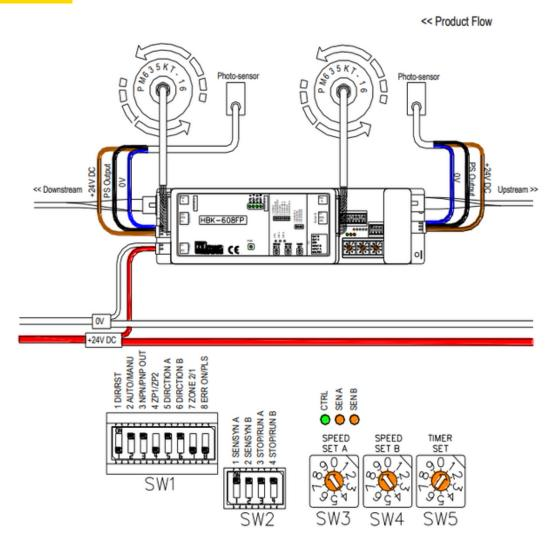
This configuration (factory set) is the standard set-up for any zone that is not specifically an infeed or discharge zone. Review page 3 for default dip switch settings.
