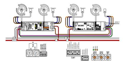
An HBK-608F can exchange handshake signals with the IB-E03B and IB-E04F. Product will accumulate at the last zone before the IB card. When sensor A is blocked on the HBK, it sends the sensor out signal to the IB. The IB then sends a force run signal to the HBK. If an HBK has an error, the error output signal is pulsed from the HBK to the IB card which can determine the error condition and bring it to upper level Ethernet communication.
