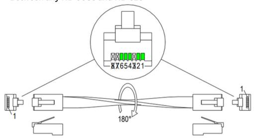
When connecting an HB-510 to an HB-508S (upstream or downstream) a special cable is recommended. This modification can be easily performed when making the communication cable. Simply disable (or cut) PINs 3, 7, and 8 according to the above diagram on the communication cable.
