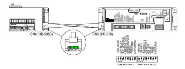
When connecting an HB-508S from CN4 to CN5 of an HB-510, DIP Switch settings must be set to ensure compatibility.
