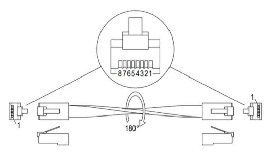
This straight through cable is intended for use between HB-510 cards. Please refer to the section **Connect to HB-508S** for further instruction when using HB-510 with HB-508S cards.
