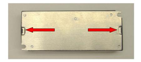
2. Change internal dip switch to appropriate setting and replace cover
